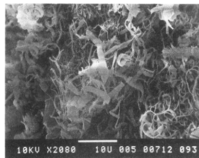
Figure 6. SEM micrograph of polyamide exp no. 4, Table 2 (the white bar represents 10 \mu\text{m} ).
